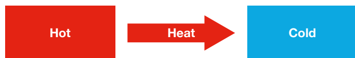
Figure 2. The second law of thermodynamics: heat will flow from a hotter body to a colder body
